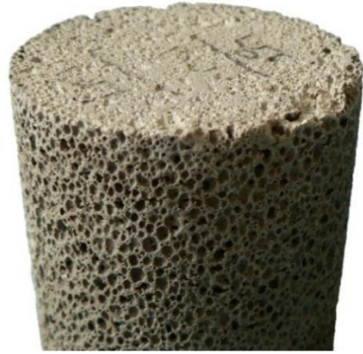
Lightweight sample from activated GBFS+Fly ash; 3,8 MPa; 722 \text{ kg}\cdot\text{m}^{-3} ; apparent porosity 72%
