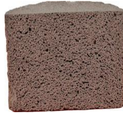
Lightweight sample from furnace slag; 3,3 MPa; 930 \text{ kg}\cdot\text{m}^{-3} ; apparent porosity 60%
