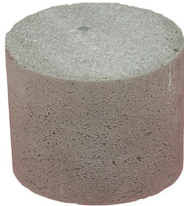
Lightweight sample from Ladle slag; 2,3 MPa; 980 \text{ kg}\cdot\text{m}^{-3} ; apparent porosity 60%
