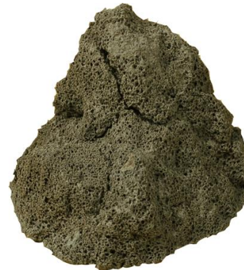
Lightweight sample from Ladle slag; 2,3 MPa; 980 \text{ kg}\cdot\text{m}^{-3} ; apparent porosity 60%
